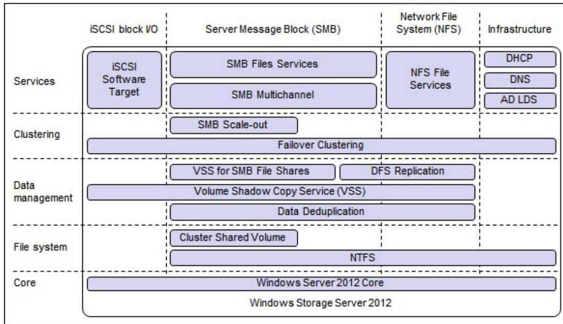
Figure 2. Windows Storage Server 2012 software components
