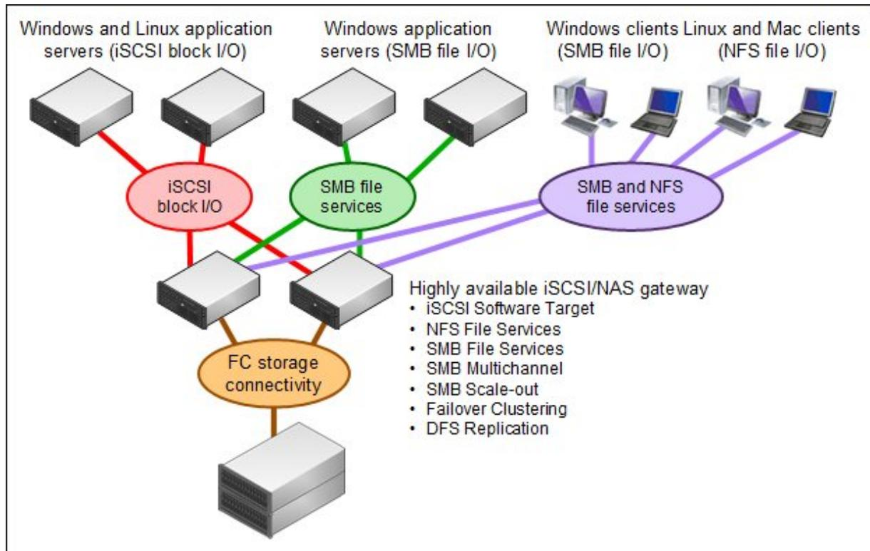
Figure 7. Highly available unified NAS gateway solution
