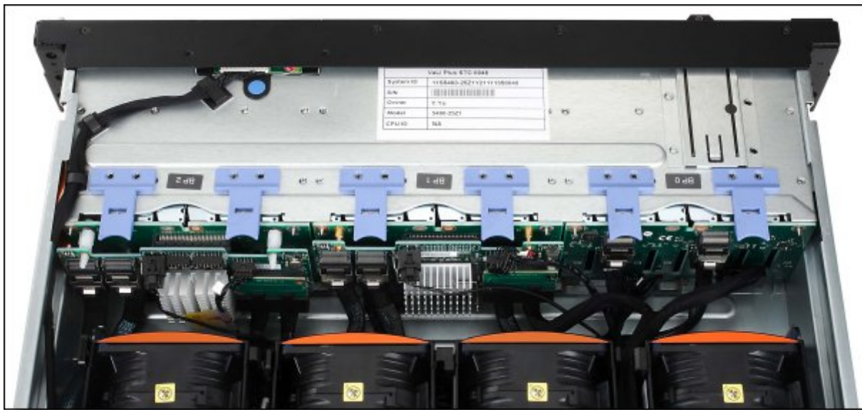
Figure 6. x3650 M4 HD Plus 8 x 2.5" HS HDD Assembly Kit with Expander installed in the server
