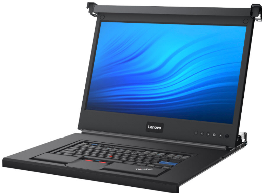
Figure 1. 1U 18.5" Standard Console (with the optional USB keyboard)
