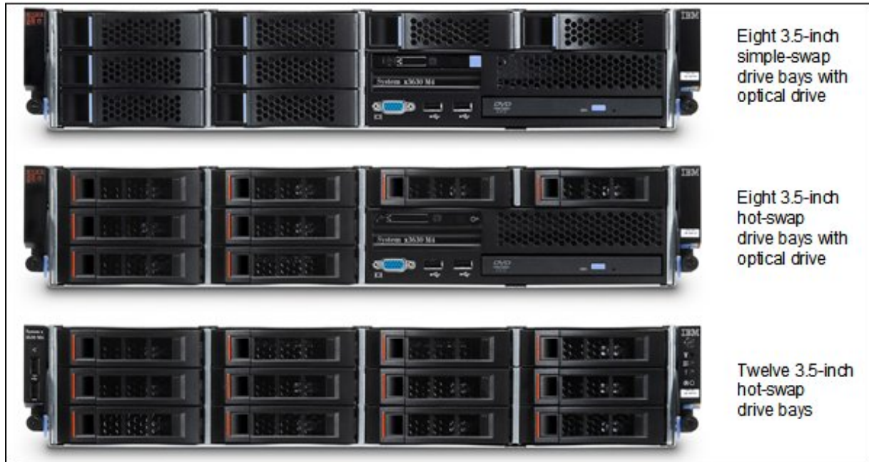
Figure 7. Internal drive configurations
