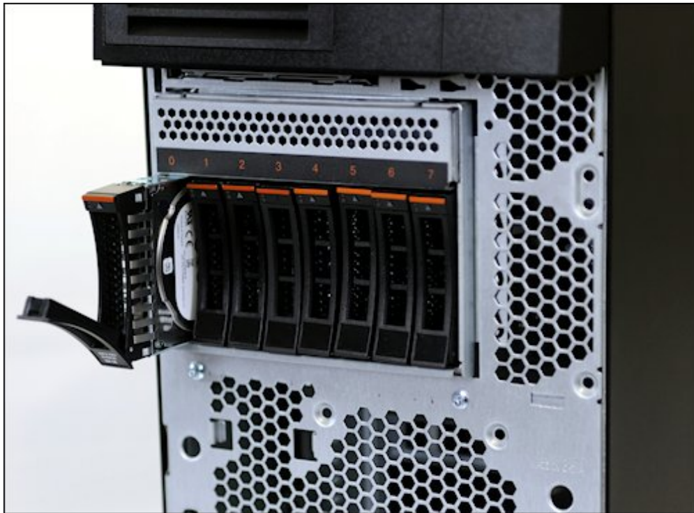
Figure 5. Hot-swap drives supported in models with hot-swap power supplies
