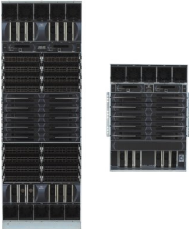
Figure 1. QLogic 12800-360 (left) and 12800-180 (right) InfiniBand switches
