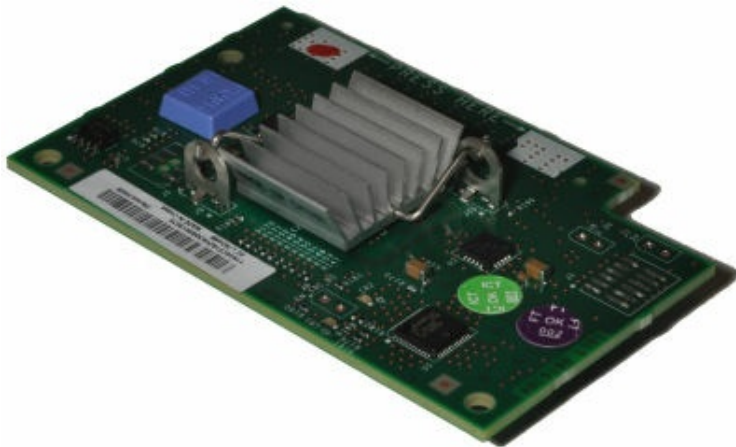
Figure 1. SAS Connectivity Card (CIOv) for BladeCenter
