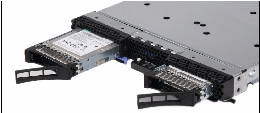
Figure 8 The HS22 showing the front hot-swap disk drive bays
