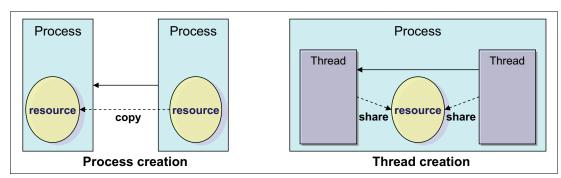
Figure 1-4 process and thread
