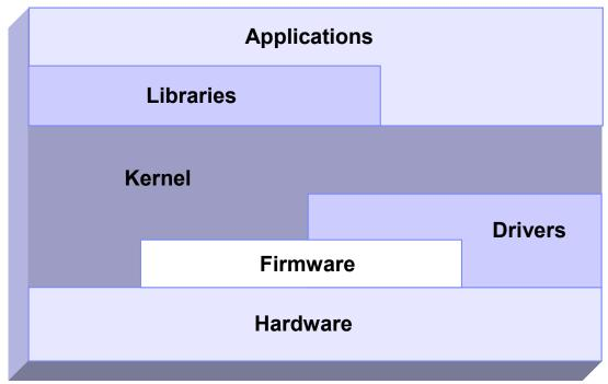
Figure 1-1 Schematic interaction of different performance components
