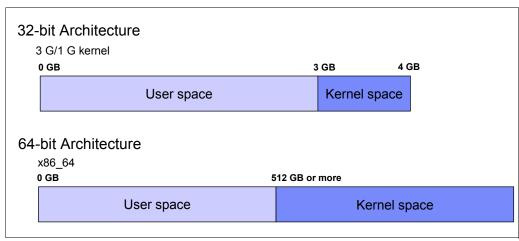
Figure 1-11 Virtual memory addressing layout for 32bit and 64-bit architecture
