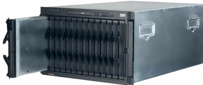
Figure 3-13 IBM BladeCenter fitted with 14 HS20 servers
