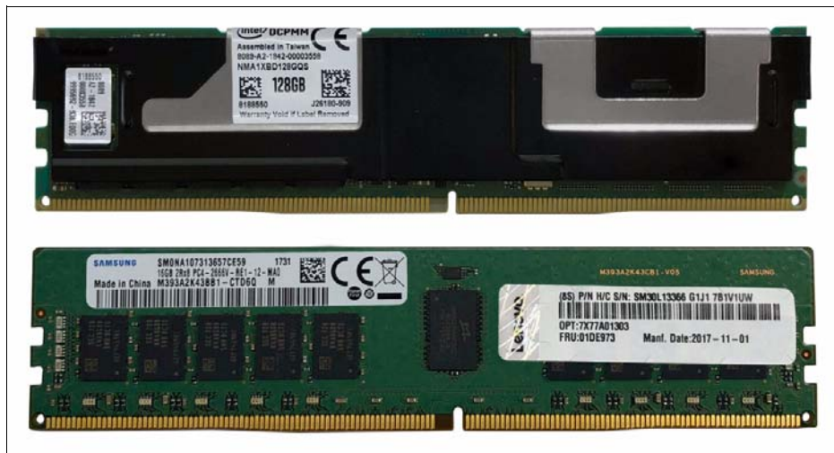
Figure 1 DCPMM (top) and a DDR4 RDIMM (bottom)
