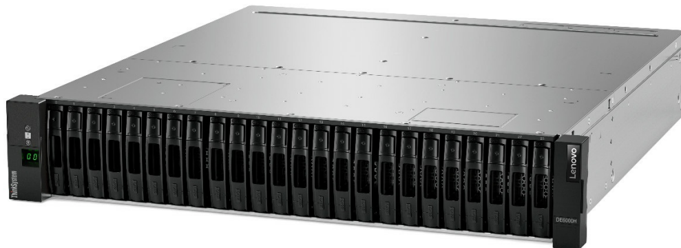
Figure 1. Lenovo ThinkSystem DE6000H Hybrid Storage Array
