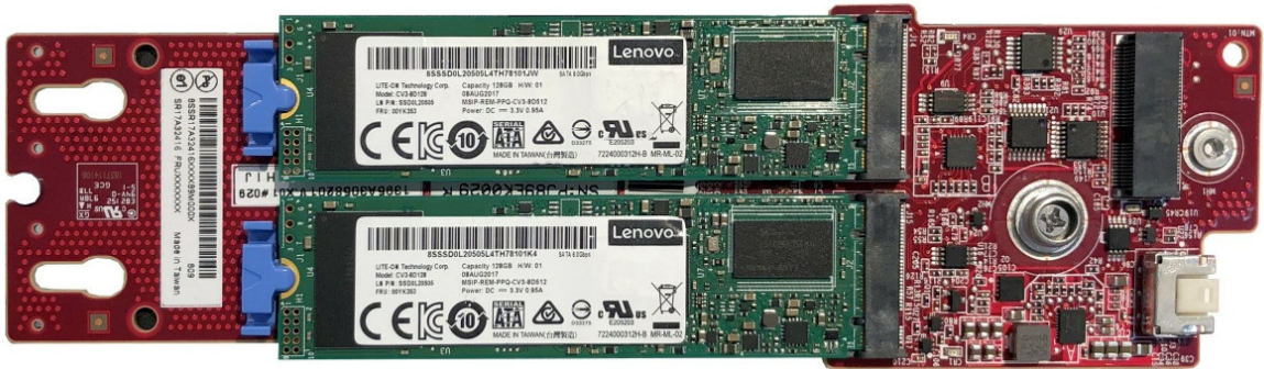
Figure 3. SATA/NVMe M.2 Module with 2 drives
