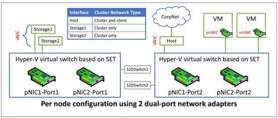
Figure 51 Diagram showing two SET teams created from two dual-port network adapters
