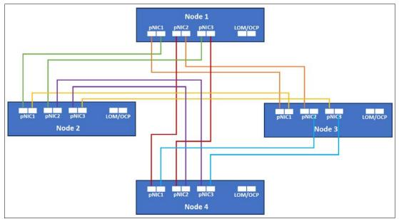
Figure 59 Four-node connectivity for direct-connected deployment sceario
