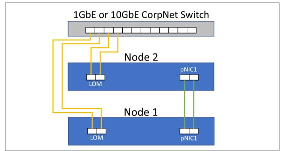
Figure 34 Two-node connectivity for direct-connected deployment scenario
