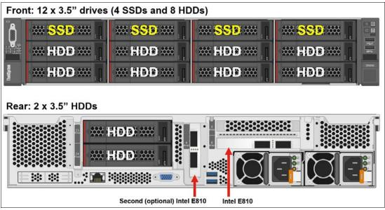
Figure 44 Lenovo ThinkSystem SR650 storage subsystem configured for iWARP
