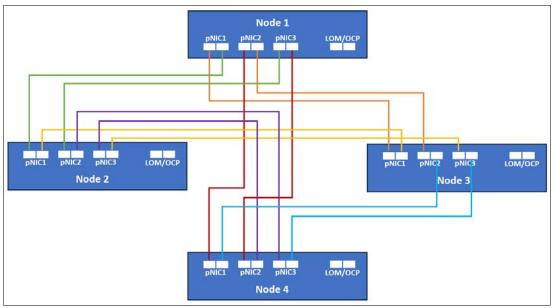
Figure 36 Four-node connectivity for direct-connected deployment scenario
