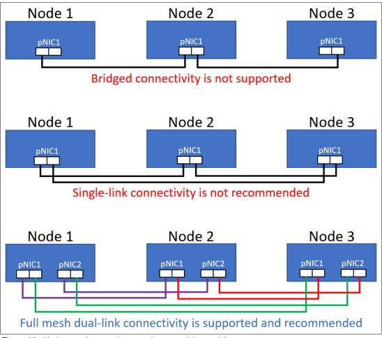
Figure 33 Various node-to-node network connectivity models
