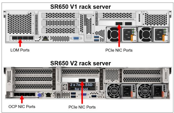
Figure 13 Placement of LOM/OCP ports in Lenovo ThinkSystem SR650 V1 and V2 rack servers
