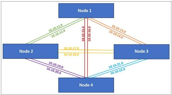
Figure 60 Simplified four-node connectivity for direct-connected scenario with example subnets shown
