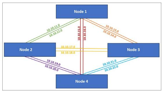
Figure 37 Simplified four-node connectivity for direct-connected scenario with example subnets shown
