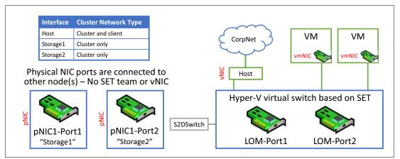
Figure 38 Two-node direct-connect network interfaces
