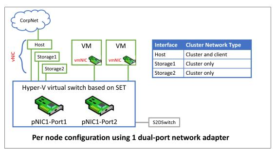
Figure 47 Diagram showing single SET team created from both ports on a single network adapter
