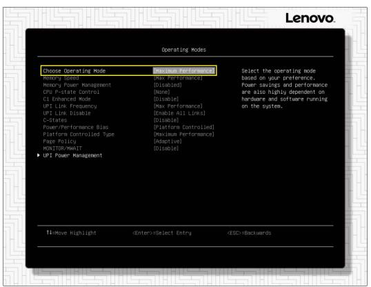
Figure 15 Text-based System Settings screen with Operating Mode set to Maximum Performance
