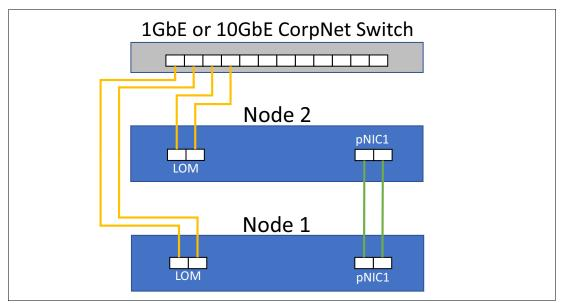
Figure 57 Two-node connectivity for direct-connected deployment scenario
