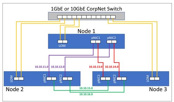
Figure 35 Three-node connectivity for direct-connected deployment scenario
