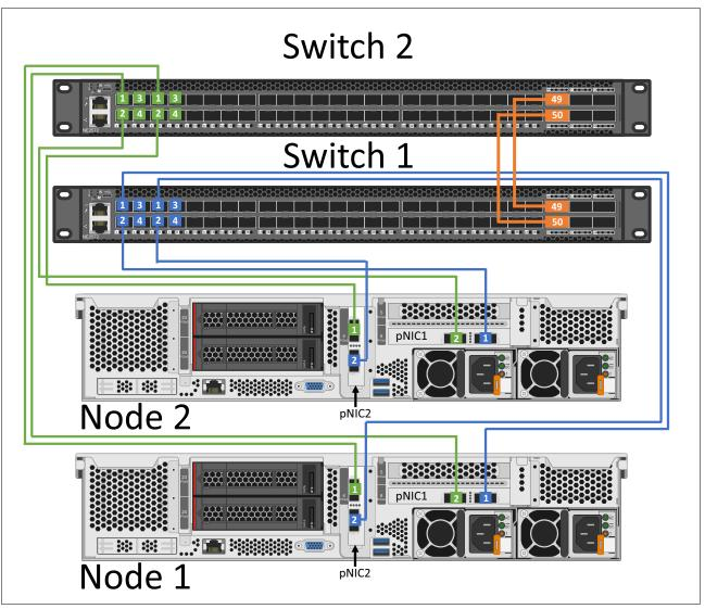
Figure 46 Switch to node connectivity using 10GbE/25GbE AOC/DAC cables and two dual-port PCIe NICs in each node
