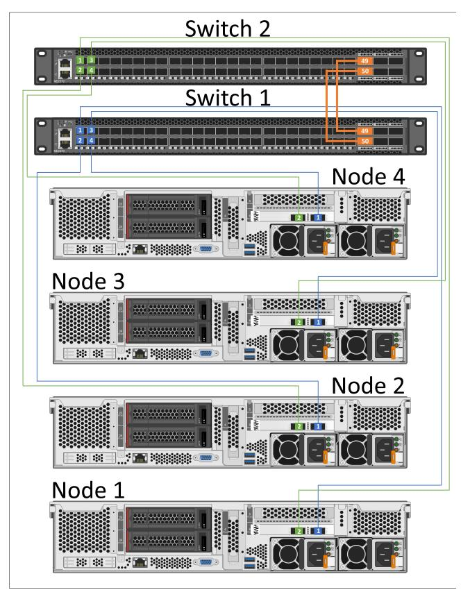
Figure 45 Switch to node connectivity using 10GbE or 25GbE AOC/DAC cables and a single dual-port NIC in each node
