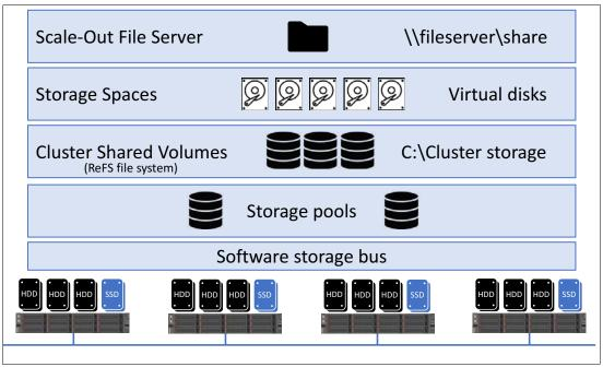
Figure 1 shows an overview of the Storage Spaces Direct stack.
