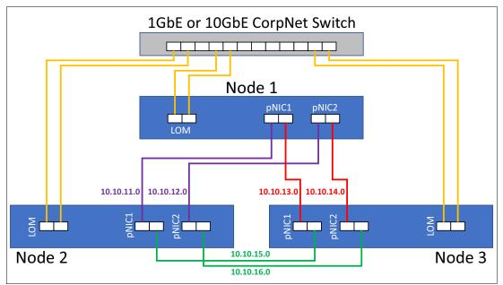
Figure 58 Three-node connectivity for direct-connected deployment scenario
