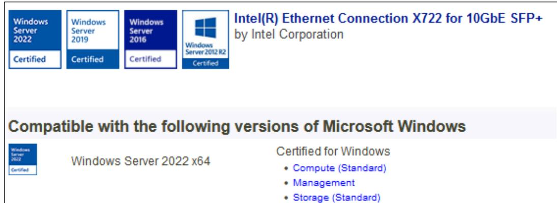
Figure 4 Microsoft HCI catalog showing Intel X722 network adapter certifications
